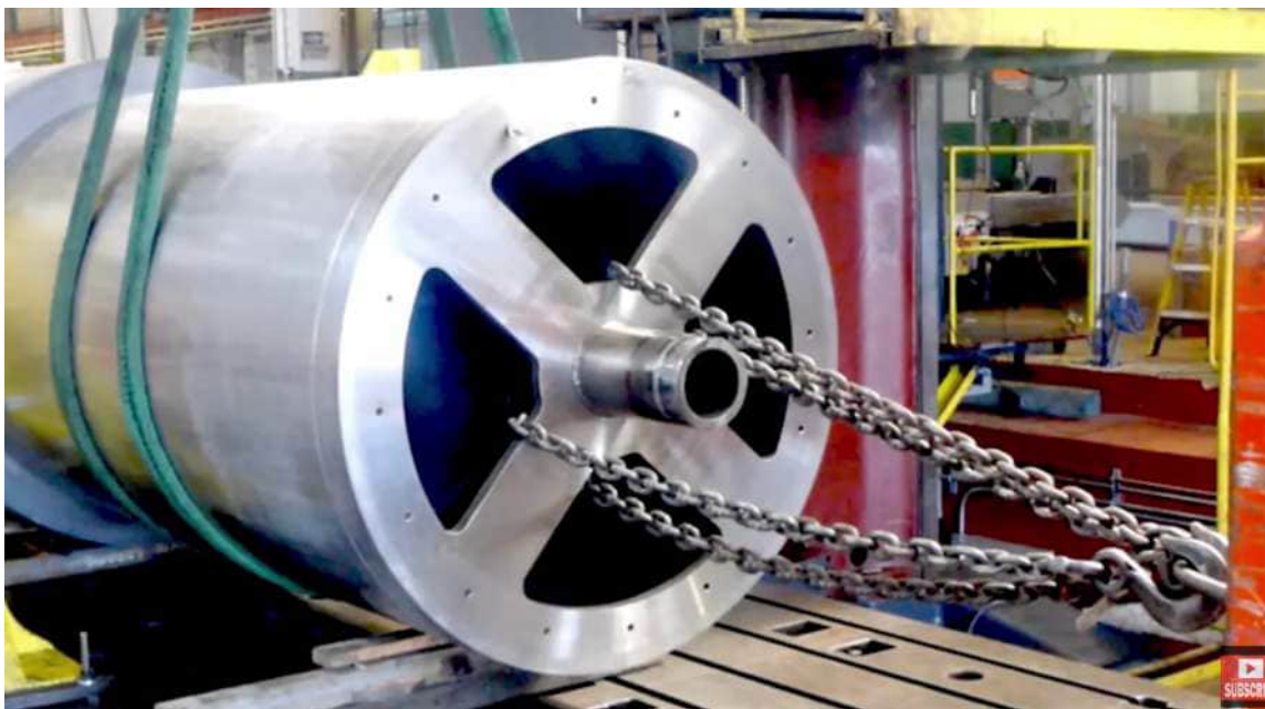
Figure: Mandrel Used to Shape Pressure Hull
