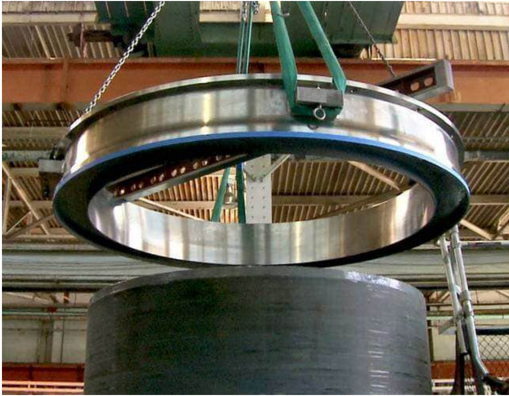
Figure: Titanium Flange Being Fitted to Carbon Fibre Hull
