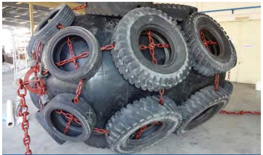
Yokohama fender repaired with Belzona
