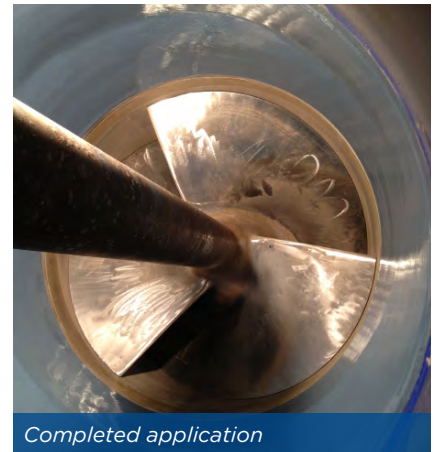
Propeller areas rebuilt and protected
